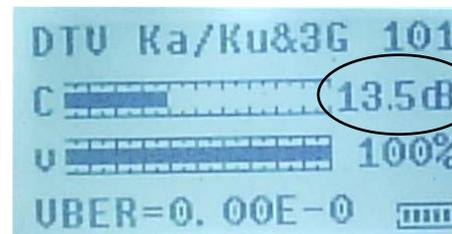
C/N ratio in dB display. Always peak this number higher for best signal quality. For example, to pass cross-pol in a 2 way system.
